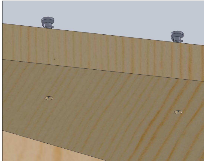
Figure 10: (1) Marking where the edge of the gusset sits. (2) Starting the screws in the back piece.
