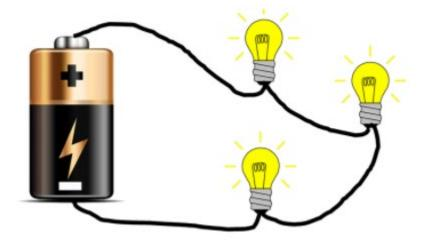
5) Each component's electrons in this circuit have their own path back to the battery. Is it series or parallel?
