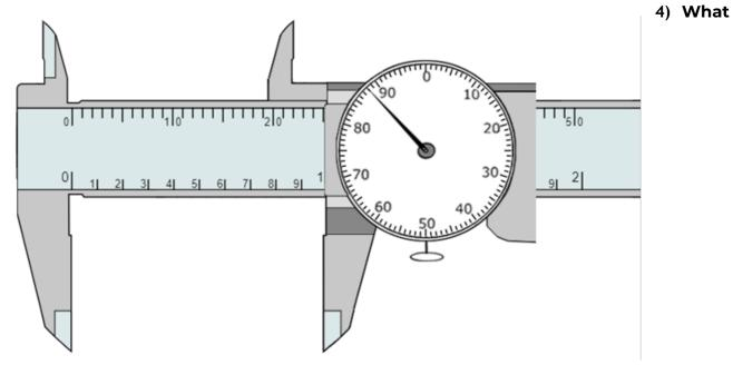
measurement is shown on this dial caliper?
